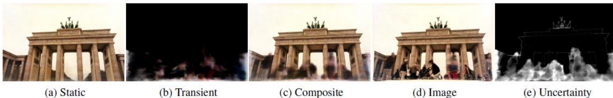
Figure 4: NeRF-W separately renders the static (a) and transient (b) elements of the scene, and then composites them (c). Training minimizes the difference between the composite and the true image (d) weighted by uncertainty (e), which is simultaneously optimized to identify and discount anomalous image regions. Photo by Flickr user vasic64 / CC BY .
