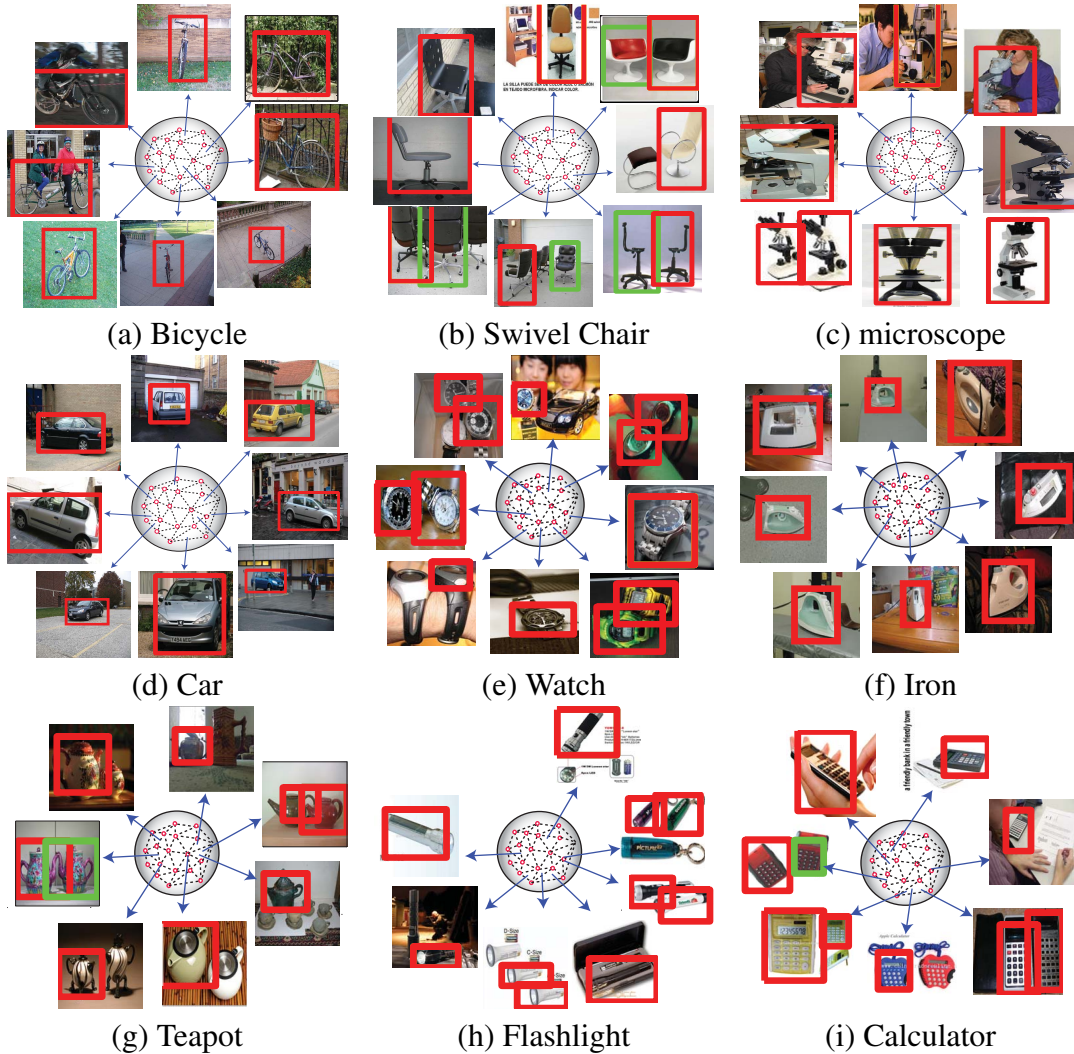
FIGURE 10.9. Examples of viewpoint estimation for bicycle [194, 57], swivel chair, microscope, car [194, 57], watch, iron, teapot, flashlight, and calculator. Blue arrows indicate the viewpoint T for the detected object (in red bounding box). Green bounding box indicates correct detections of the objects, but in a different viewpoint.
