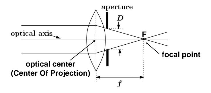
A lens focuses parallel rays onto a single focal point
