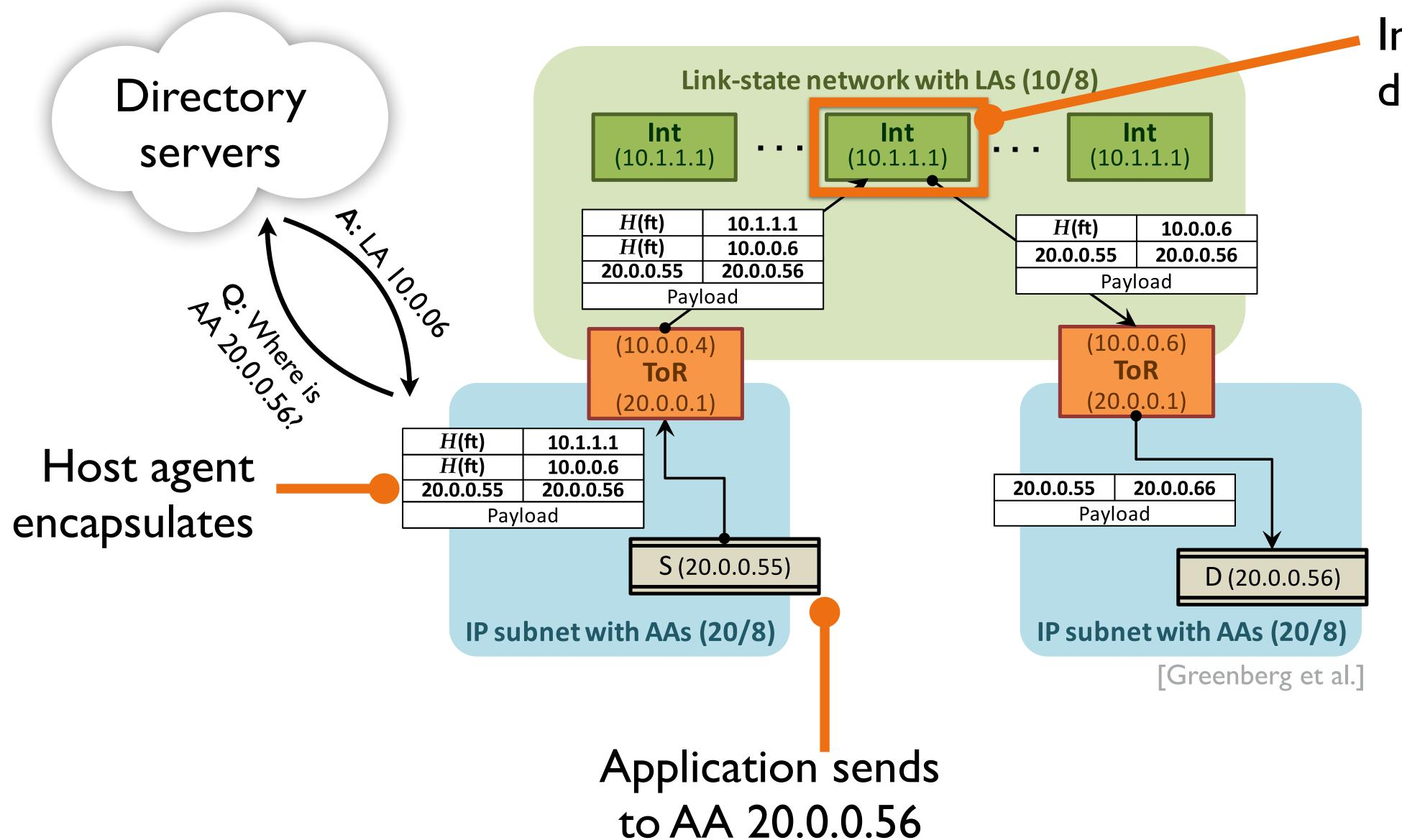
Intermediate switch decapsulates
