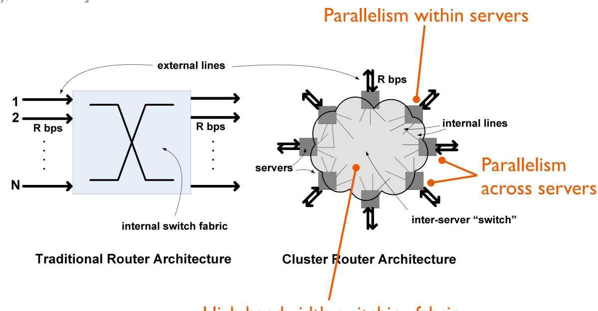
High bandwidth switching fabric built from commodity hardware
