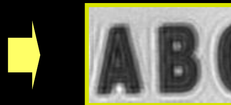
Ringing with the traditional Richardson-Lucy deconvolution algorithm
