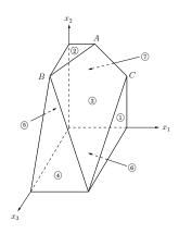
$$\begin{array}{cccc} \max & x_1 + 6x_2 + 13x_3 \\ & x_1 \leq 200 & & \textcircled{1} \\ & x_2 \leq 300 & & \textcircled{2} \\ & x_1 + x_2 + x_3 \leq 400 & & \textcircled{3} \\ & x_2 + 3x_3 \leq 600 & & \textcircled{4} \\ & x_1 \geq 0 & & \textcircled{5} \\ & x_2 \geq 0 & & \textcircled{6} \\ & x_3 \geq 0 & & \textcircled{7} \end{array}$$
