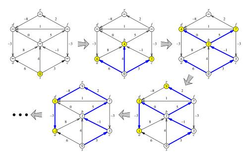
**Figure 8.5.** Four phases of Bellman-Ford run on a directed graph with negative edges. Nodes are taken from the queue in the order  $s \diamond a \ b \ c \diamond d \ f \ b \diamond a \ e \ d \diamond d \ a \diamond \diamond$ , where  $\diamond$  is the end-of-phase token. Shaded vertices are in the queue at the end of each phase. The bold edges describe the evolving shortest path tree.
