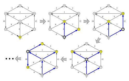
**Figure 8.4.** Four phases of Dijkstra's algorithm run on a graph with no negative edges. At each phase, the shaded vertices are in the heap, and the bold vertex has just been scanned. The bold edges describe the evolving shortest path tree.
