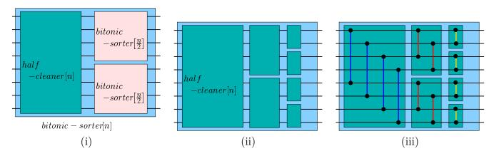
Figure 9.5: Depicted are the (i) recursive construction of BitonicSorter[n], (ii) opening up the recursive construction, and (iii) the resulting comparison network.
