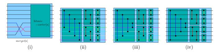
Figure 9.6: (i) Merger via flipping the lines of bitonic sorter. (ii) A BitonicSorter. (ii) The Merger after we "physically" flip the lines, and (iv) An equivalent drawing of the resulting Merger.
