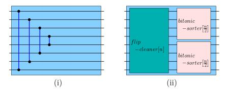
Figure 9.7: (i) FlipCleaner [n], and (ii) Merger [n] described using FlipCleaner.
