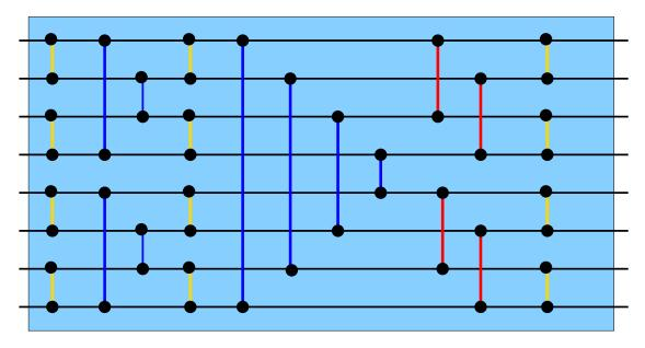
Figure 9.9: The resulting sorting network for input of size n: Sorter[8].
