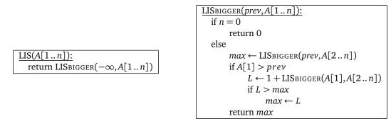
The running time of this algorithm satisfies the recurrence  $T(n) \le 2T(n-1) + O(1)$ , which as usual implies that  $T(n) = O(2^n)$ . We really shouldn't be surprised by this running time; in the worst case, the algorithm examines each of the  $2^n$  subsequences of the input array.
