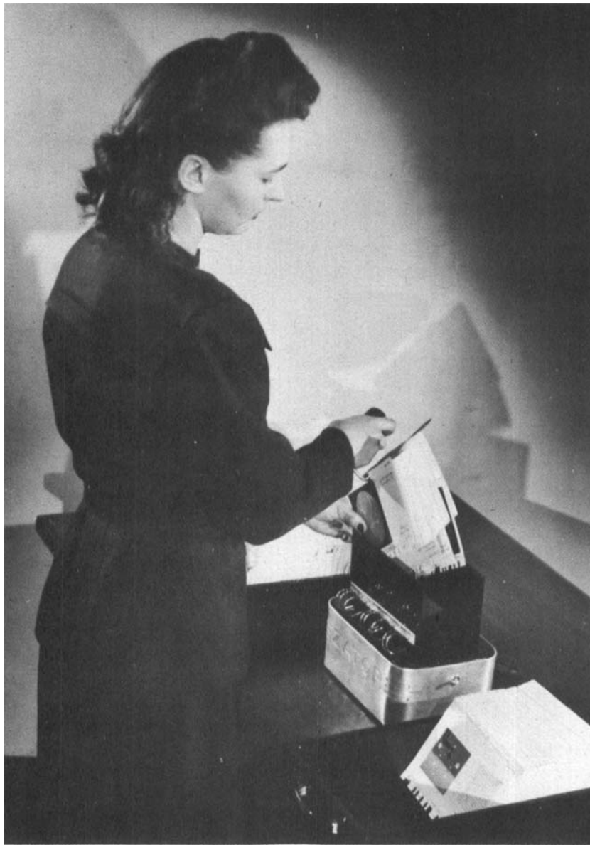
Fig. 2. THE ZATOR SELECTOR, capable of sorting edge notched Zatorcards at the rate of 800 cards per minute. The black box-like portion of the Zator Selector is vibrated by a motor in the base. At the bottom of the box, a row of holes allows pins to be inserted to form the selective grid pattern. For selection, a pack of Zatorcards is placed notched edge down on the vibrating grid. The rejected cards are those whose edge notches do not fit the pattern of the grid; hence they are supported on top of the grid. The edge notches of the accepted cards fit the grid and the cards drop down through the grid to a distance equal to the depth of the notches. In this way, the accepted cards are offset slightly below the rejected cards. To separate the rejected cards from the accepted cards the operator spears the pack of rejected cards through the small hole on the edge opposite the notches and lifts the pack out. The accepted cards, being offset below the rejected cards, are not engaged by the spearing tool; they drop out from the pack onto the table.
