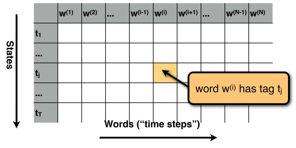
We use a N×T table ("**trellis**") to keep track of the HMM. The HMM can assign one of the T tags to each of the N words.
