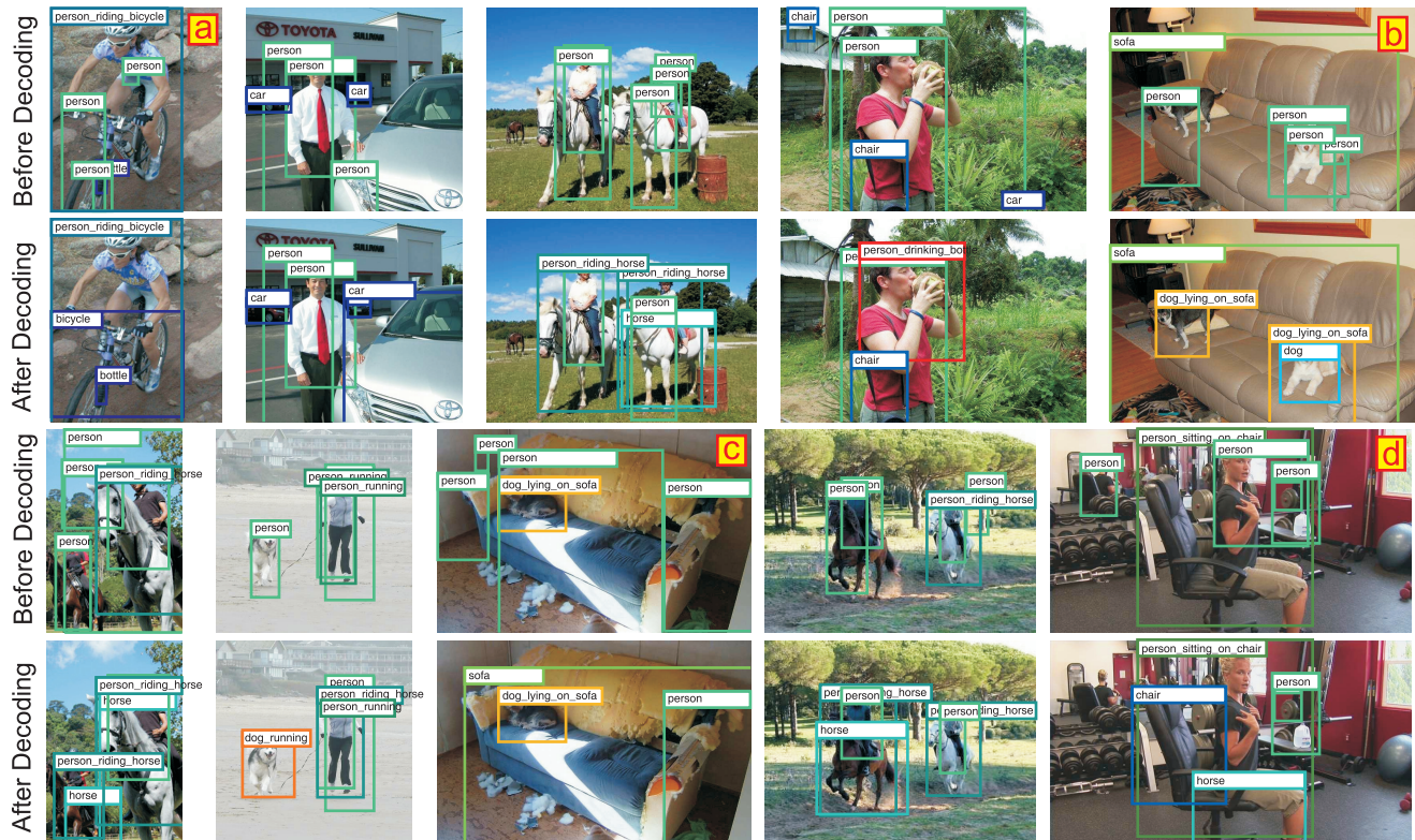
Figure 6. Rows 1 and 2 depicts our results before and after decoding, respectively. The same applies to rows 3 and 4. For example, in image “a”, our decoding boosts the confidence of the bicycle classifier and suppresses the confidences of wrong person detections using a reliable “person riding bicycle” detection. In image “c”, a confident “dog lying on sofa” detector improves the confidence of the sofa detection and decreases the confidences of wrong person detections. In image “d”, the “person sitting on chair” detector increases the confidence of the chair detection. Our decoding shows that visual phrases help object detection and vice versa. In image “b”, the confident sofa detection boosts the confidence of “dog lying on sofa” detection.
