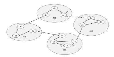
Consider the network shown above. Suppose AS3 and AS2 are running OSPF for their intra-AS routing protocol. Suppose AS1 and AS4 are running RIP for their intra-AS routing protocol. Suppose eBGP and iBGP are used for the inter-AS routing protocol. Suppose there is no physical link between AS2 and AS4 (ignore the dashed line).
