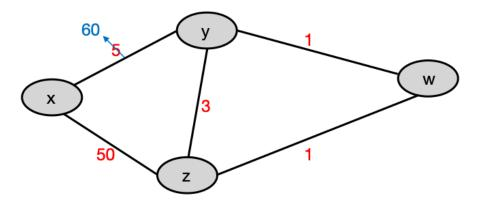
Initially, the cost of different links are: c(x,y) = 5, c(x,z) = 50, c(y,z) = 3, c(y,w) = 1, c(z,w) = 1
