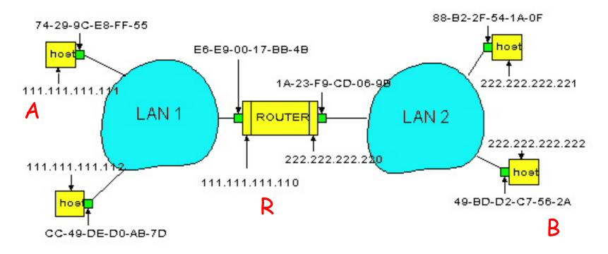
Two ARP tables in router R, one for each IP network (LAN)
