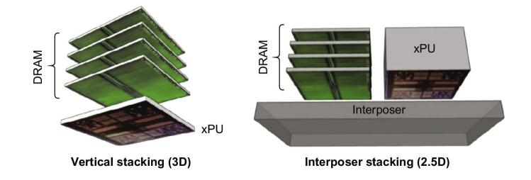
Figure 2.7 Two forms of die stacking. The 2.5D form is available now. 3D stacking is under development and faces heat management challenges due to the CPU.
