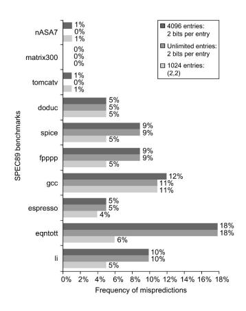
**Figure 3.3 Comparison of 2-bit predictors.** A noncorrelating predictor for 4096 bits is first, followed by a noncorrelating 2-bit predictor with unlimited entries and a 2-bit predictor with 2 bits of global history and a total of 1024 entries. Although these data are for an older version of SPEC, data for more recent SPEC benchmarks would show similar differences in accuracy.
