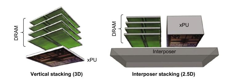
Figure 2.7 Two forms of die stacking. The 2.5D form is available now. 3D stacking is under development and faces heat management challenges due to the CPU.
