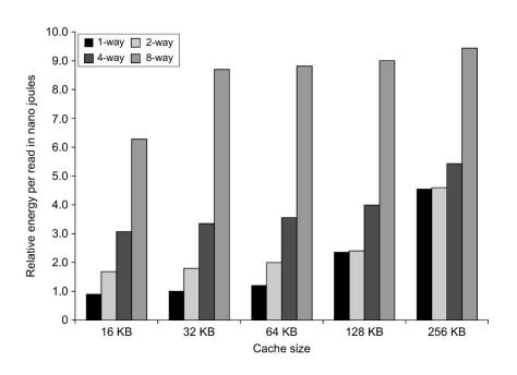
**Figure 2.9 Energy consumption per read increases as cache size and associativity are increased.** As in the previous figure, CACTI is used for the modeling with the same technology parameters. The large penalty for eight-way set associative caches is due to the cost of reading out eight tags and the corresponding data in parallel.
