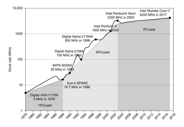
*Figure 1.11 Growth in clock rate of microprocessors in Figure 1.1.* Between 1978 and 1986, the clock rate improved less than 15% per year while performance improved by 22% per year. During the "renaissance period" of 52% performance improvement per year between 1986 and 2003, clock rates shot up almost 40% per year. Since then, the clock rate has been nearly flat, growing at less than 2% per year, while single processor performance improved recently at just 3.5% per year.
