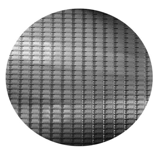
Figure 1.15 This 300 mm wafer contains 280 full Sandy Bridge dies, each 20.7 by 10.5 mm in a 32 nm process. (Sandy Bridge is Intel's successor to Nehalem used in the Core i7.) At 216 mm2, the formula for dies per wafer estimates 282. (Courtesy Intel.)
