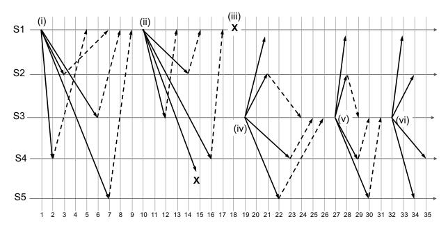
It demonstrates a series of events / message exchanges in a Raft cluster. The numbers at the bottom show the real time. Initially all servers start in follower state in term 0. The following key events occur as indicated in the figure:
