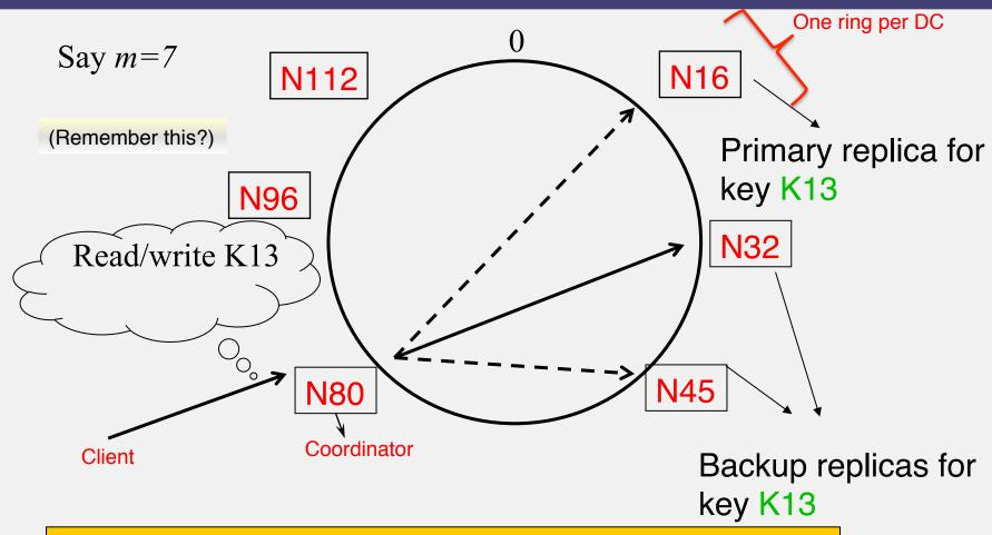
Cassandra uses a Ring-based DHT but without finger tables or routing Key -> server mapping is the "Partitioner"
