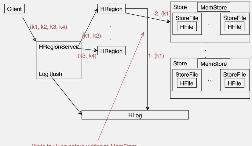
Write to HLog <u>before</u> writing to MemStore Helps recover from failure by replaying Hlog.
