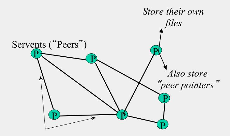
Connected in an **overlay** graph
