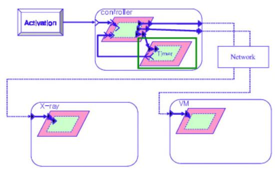
Architecture #1: Master controller on a Windows server orchestrates ventilator and X-ray machine actions over a network. Controllers tells machines to stop and re-start, and ensures that ventilator is not off too long. Comments?
