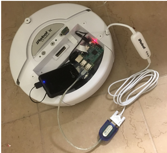
Fig 6.2(a) Connecting iRobot to Pi using the Serial connector and USB-Serial Adapter
