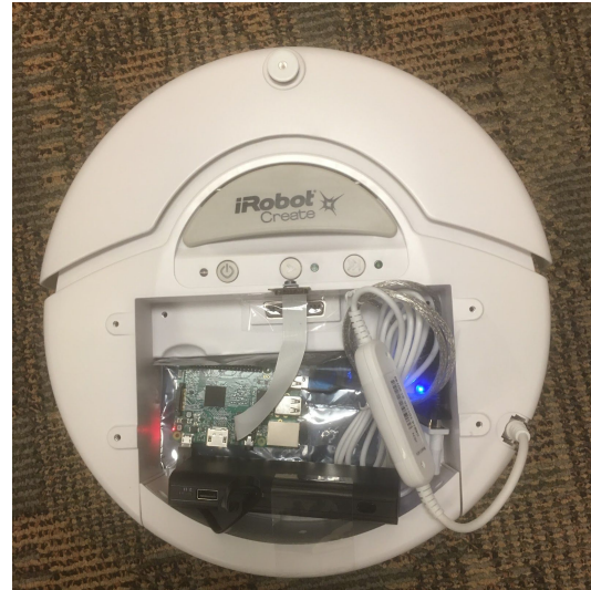
Fig 6.2(b) A completely mobile assembly of the iRobot and Raspberry Pi
