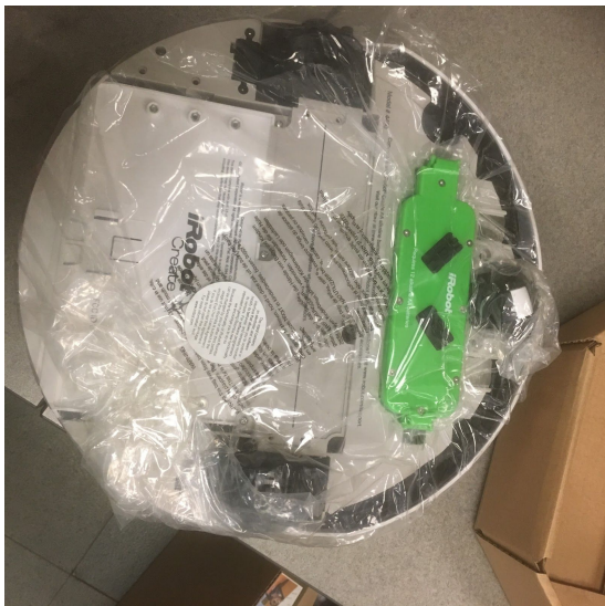
Fig 6.1(a) iRobot create may initially contain a green colored AA battery container.
