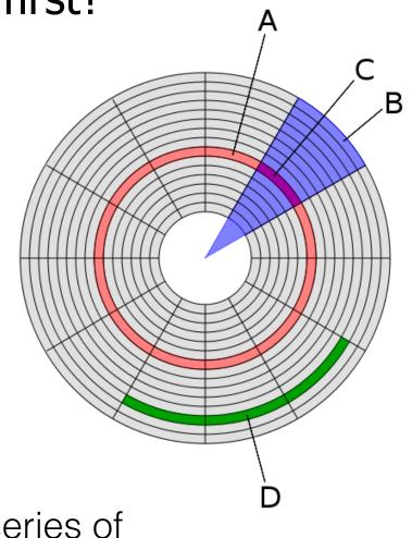
**Disk Scheduling Decision** — Given a series of access requests, on which track should the disk arm be placed next to maximize fairness, throughput, etc?
