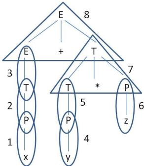
(b) (10 pts) Based on the tree above, fill in the following table, giving parse actions under various combinations of stack and lookahead symbol; the actions can be *shift*, *reduce by a given production*, and *accept*. There are no *reject* actions here; we filled in the first row.
