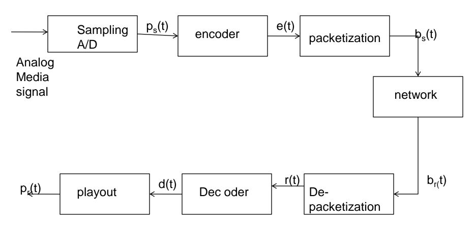
p(t) – amount of captured/playout bits its at time t; e(t), d(t) amount of encoded/decoded bits at time t; b(t) - amount of clustered bits at time t
