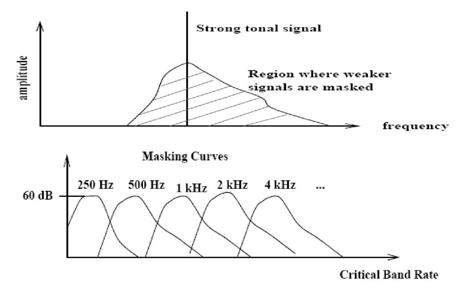
MPEG/audio divides audio signal into frequency sub-bands that approximate critical bands. Then we quantize each sub-band according to the audibility of quantization noise within the band
