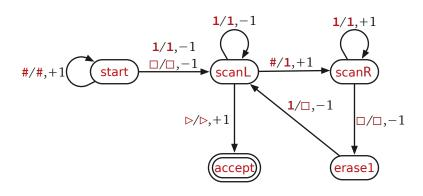
**3** On input  $\#1^n$ , for any non-negative integer *n*, write  $\#1^{2n}$  on the tape and accept. (Hint: Modify the Turing machine from problem 1.)
