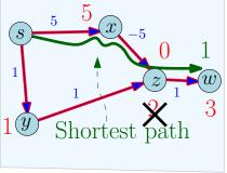
False assumption: Dijkstra's algorithm is based on the assumption that if  $s = v_0 \rightarrow v_1 \rightarrow v_2 \dots \rightarrow v_k$  is a shortest path from s to  $v_k$  then  $dist(s, v_i) \leq dist(s, v_{i+1})$  for  $0 \leq i < k$ . Holds true only for non-negative edge lengths.
