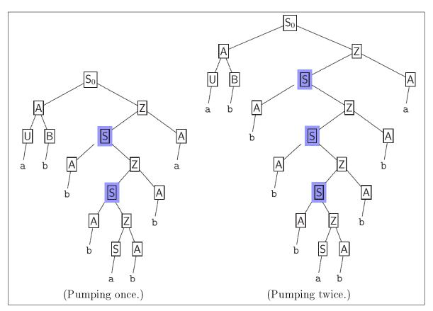
Naturally, we can repeat this pumping operation (cutting and pasting a subtree) as many times as want, see for example Figure 1. In particular, we get that the word  $abb^iab^ia$ , for any i, is in the language of the grammar (G5). Notice that unlike the pumping lemma for regular languages, here the repetition happens in two places in the string. We claim that such a repetition (in two places) in the word must happen for any context free language, once we take a word which is sufficiently long.
