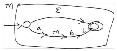
**Example 2:** Let us design a recursive automaton for the language  $L = \{w \in \{a, b, c\}^* \mid w \text{ is a palindrome }\}$ . Thinking recursively, the smallest palindromes are  $\epsilon$ , a, b, c, and we can construct a longer palindrome by generating awa, bwb, cwc, where w is a smaller palindrome. This give us the following recursive automaton:
