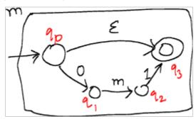
Why? The recursive automaton consists of single module, which is also the main module. The module either accepts  $\epsilon$ , or reads 0, calls itself, and after returning from the call, reads 1 and reaches a final state (at which point it can return if it was called). In order to accept, we require the run to return from all calls and reach the final state of module main.
