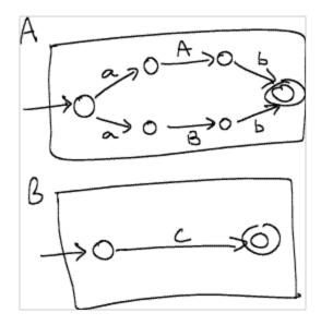
Formally, let  $G = (V, \Sigma, R, S)$  be a context free grammar. Let  $A_G = (M, main, \{(Q_m, \Sigma \cup M, \delta_m, q_0^m, F_m)\}_{m \in M})$  where M = V, main = S and for each  $X \in M = V$ , let  $\langle Q_m, \Sigma \cup M, \delta_m, q_0^m, F_m \rangle$  be an NFA that accepts the (finite, and hence) regular language  $L_X = \{w | (X \to w) \in R\}$ . Then  $L(G) = L(A_G)$ .
