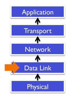
The **Data Link Layer** sends and receives packets on a transmission medium.
