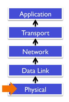
The **Physical Layer** provides hardware-specific details on how to transmit a 0 vs. 1.
