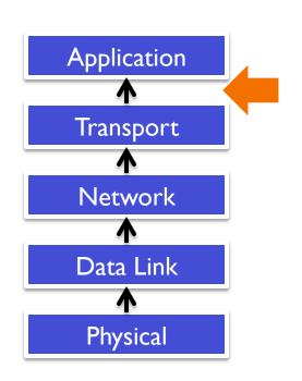
Most commonly, we write applications using an interface to the transport layer
