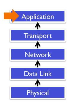
The **Application Layer** refers to any communication software and procedures for particular applications.
