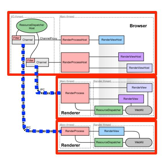
A named pipe is allocated for each renderer process for communication with the browser process
