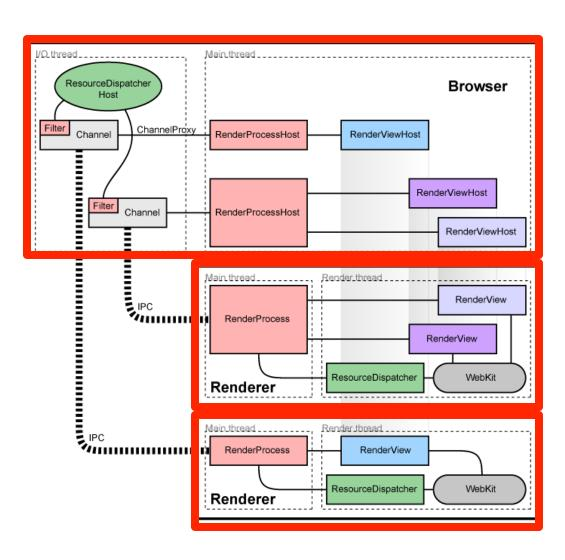
Separate processes for browser tabs to protect the overall application from bugs and glitches in the rendering engine
