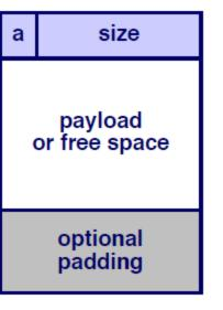
a = 1: block is allocated a = 0: block is free
