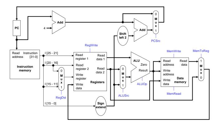
2. Extend the datapath shown below to support load upper immediate lui. Recall that lui is an I-type instruction that performs the following operation:
