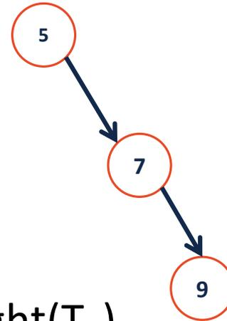
Height balance:  $b = \text{height}(T_L) - \text{height}(T_R)$
