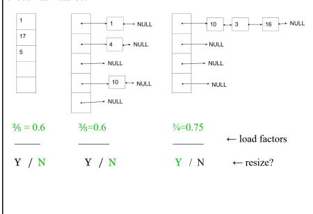
**Exercise 3.2:** Suppose that our hash function for the table below is a simple mod function:  $h(x) = x \mod TABLE\_SIZE$  and we use linear probing to resolve collisions. Our load factor threshold is 0.7, so we will need to resize the table. Draw the new resized table.
