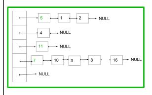
Exercise 2.2: What is the worst possible runtime for the insert() function if we are using separate chaining to resolve collisions? What about the worst possible runtime for the find() function? insert() will always be O(1) because we insert into the head of the linked list. find() however can be O(n) at the worst.
