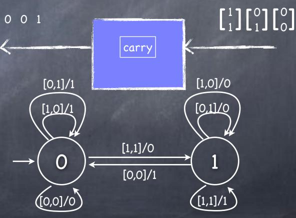
Transition function: maps (state,input) pairs to (state,output) pairs
