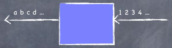
The system's output at any moment depends not only on the "current" input but also on what the system "remembers" about the past
