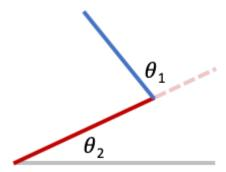
The first (blue) segment has length  $l_1$ . It is bent relative to the second segment at angle  $\theta_1$ . (We always define this angle as a counter-clockwise rotation away from the previous segment, which we extended as a faint dashed line.) The second (red) segment has length  $l_2$  and is rotated at angle  $\theta_2$  from the horizontal axis.
