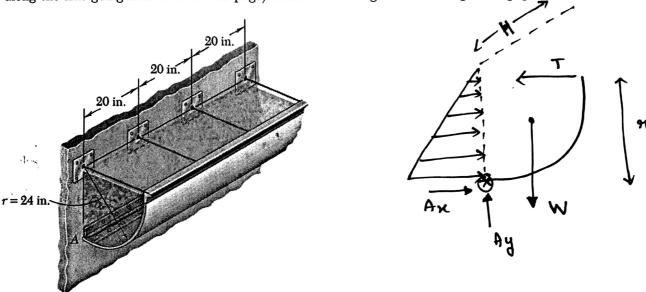
b) Calculate the horizontal component of the equivalent hydrostatic pressure force on the trough, and the corresponding  $\bar{y}$  location measured from A.
