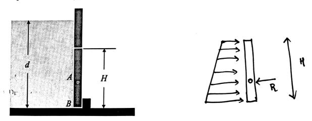
if the equivalent fluid pressure acts above 'A', then there will be a clockwise moment about A which notates the plate and opens the valve.
