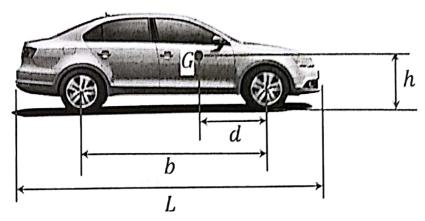
We want to consider what the largest slopes — pointing uphill and downhill that this vehicle can handle when placed on (a) dry pavement, and (b) icy pavement. For everything ahead, we will simplify the problem by considering it in 2D: so the front wheels act together and the rear wheels act together.
