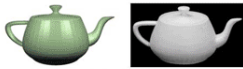
Figure 2. A closed polygonal model of the Utah teapot (left) and the resulting plastic teapot created by rapid prototyping (right).
