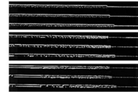
Fig. 7. Boiling CO 2 in micro-channel: upper to lower: 15 °C, 5 °C, -25 °C.
