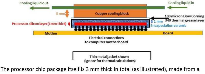
1 mm-thick active silicon layer centrally-sandwiched with 1 mm of ceramic encapsulant above & below it. The ceramic fill has a thermal conductivity of 200 Wm<sup>-1</sup>.K<sup>-1</sup>. 4 Physics 524: Survey of Instrumentation & Laboratory Techniques:
