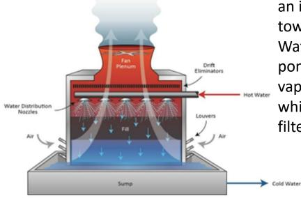
Water cooling tower, typically used at power stations and big industrial plants & data centers. Secondary hot water from a heat exchanger cooling an industrial process is pumped to the top of the tower and sprayed into a counter flow of air. Water is thus cooled and collected in the bottom pond. The circuit is open, some water escapes as vapour and must be replenished,
