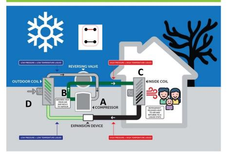
The special component: a (usually electric – driven) fluid "4-way switch"
