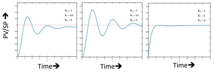
Screenshots (from https://en.wikipedia.org/wiki/File:PID Compensation Animated.gif) the time-dependent response of the measured value (blue curve) of a process variable (PV) following a step change in setpoint (SP) when regulated by an automatic learning-mode PID algorithm. **x-axis**: time (arbitrary units): **y axis**: measured value of the process value relative to the new set point (taken to be 1).
