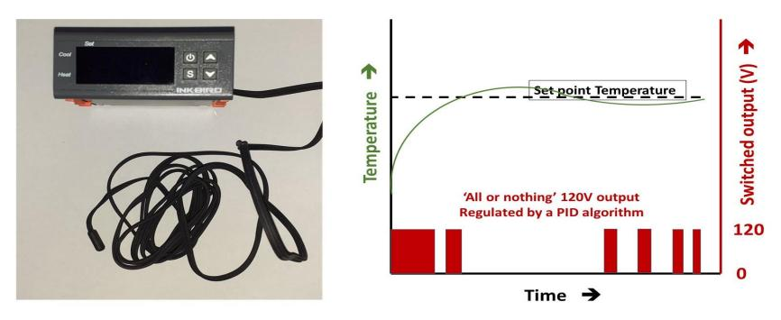
Inexpensive digital controller with NTC thermistor & <u>P</u>ulse <u>W</u>idth <u>M</u>odulated ("All or Nothing") relay output driven by a PID (<u>P</u>roportional, <u>I</u>ntegral and <u>D</u>erivative algorithm)
