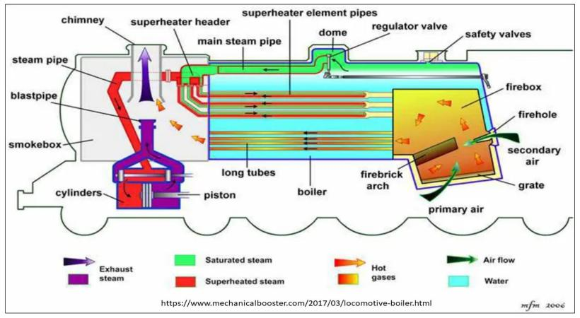
Another form of evaporative heat exchanger: the steam locomotive:
