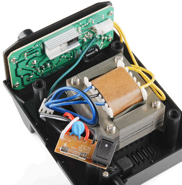
The insides of a soldering iron base
