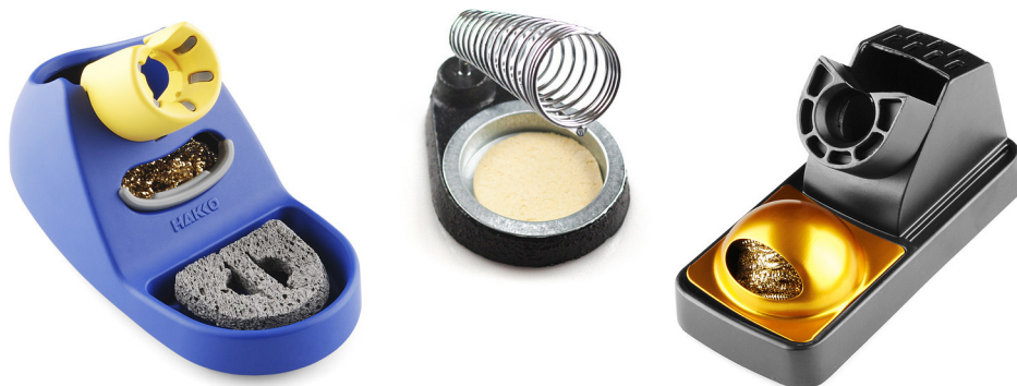
Different types of iron cradles. Notice some allow for a regular sponge while others hold a brass sponge.
