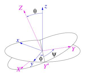
Euler angles: we first rotate the ball through an angle  $\phi$  about the z axis, thus taking  $y \to Y'$ , then through  $\theta$  about Y', and finally through  $\psi$  about Z, so taking  $Y' \to Y$ .
