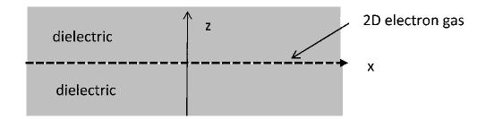
A two-dimensional gas of electrons is confined at the z=0 interface between two semiinfinite dielectric slabs. Each slab has dielectric constant  $\varepsilon$ . A perturbation of the electron charge-density propagates as a wave through the electron gas. The surface-charge density on the interface is therefore given by  $\sigma(x,t) = \sigma_0 + \sigma_1(x,t)$ , where  $\sigma_0$  is constant and the small-amplitude perturbation  $\sigma_1$  takes the form
