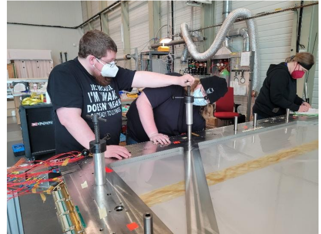
Replacing 20 \mu m W/Au anodes
